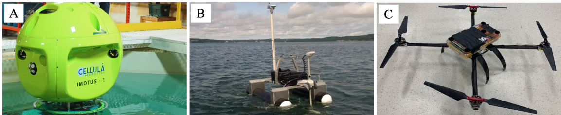
Figure 3.9: (a) IMOTUS hover-capable unmanned underwater vehicle, (b) Intelligent Systems Laboratory's high buoyancy unmanned surface vehicle, approaching the camera, and (c) unmanned aerial vehicle, Pelican, designed to be marinized and networked through the motion capture system and controlled through mRobot [2].
