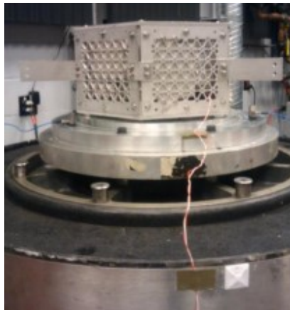
Figure 4.2 Kind of CubeSat mounted to the shaker table [14].
