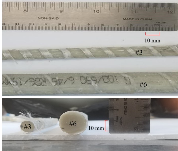
Fig. 2. Bar size and bar cross-sections.
