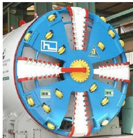
Figure 2- 7: Slurry face boring machine (SFM) (from Herrenknecht)
