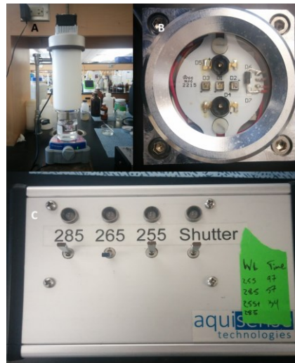
Figure 4.3: A) UV-LED collimated beam apparatus, B) UV-LED light sources and C) UV-LED collimator shutter control box
