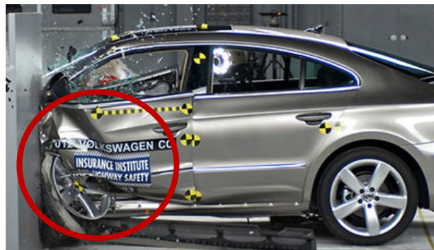
Figure 1-2. Small overlap frontal crash test of a 2012 Volkswagen CC 1 . Buckling of the front door is highlighted.
