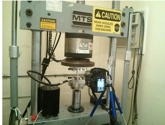
Figure 3-1. Experimental set up: MTS testing machine with a specimen in test-fixture and the camera used for recording the response.
