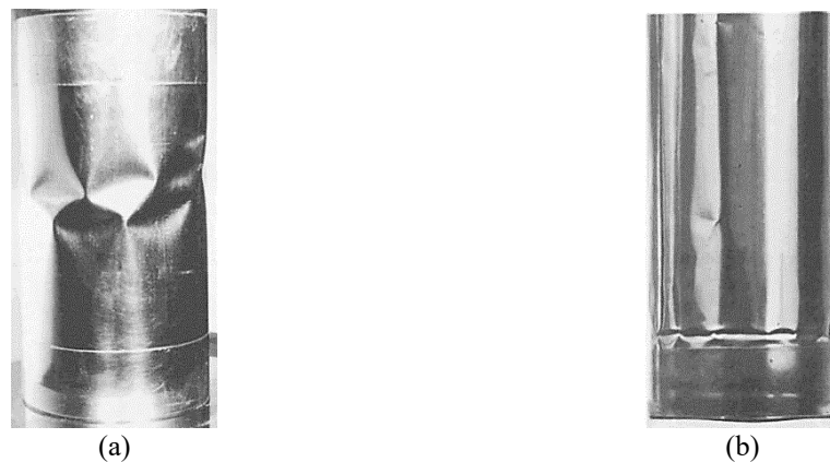
Figure 1-4. Comparison between (a) static and (b) dynamic buckling patterns for a thin cylindrical shell (Lindberg & Florence, 1987).
