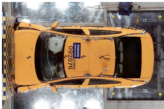
Figure 10-1. Top view of a full-frontal crash test (VolvoCars, 2019).
