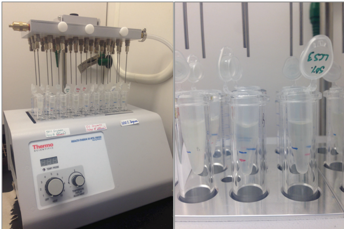
Figure A-2. Nitrogen stream concentration of the three separate batches of serum samples (left) and markings showing different sample concentration volumes (right).
