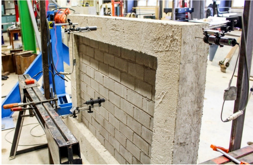
Figure 3.2. Out-of-plane LVDTs and LVDT 1
