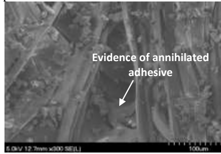
(c) Specimen subjected to 450 cycles
