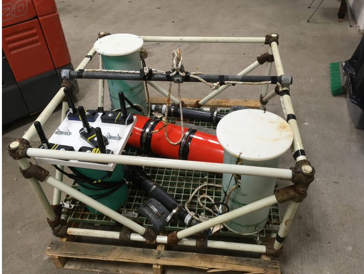
Figure 3.13: Cage used to deploy receiver at the Fundy Ocean bed
