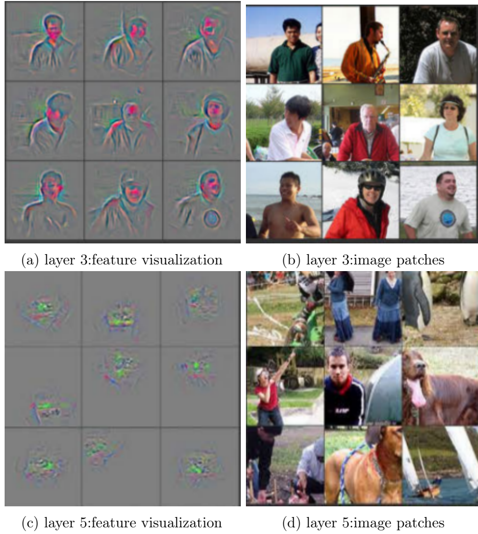
Figure 2.5: Feature visualizations and image patches of the top 9 stimuli that excite a specific feature map at layer 3 and 5 for a trained neural network from [187].
