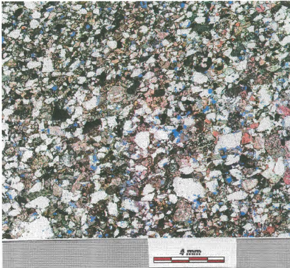
Figure 4.4 Poorly sorted sandstone with irregular laminae of finer grained material (Hunt Oil, 1998)
