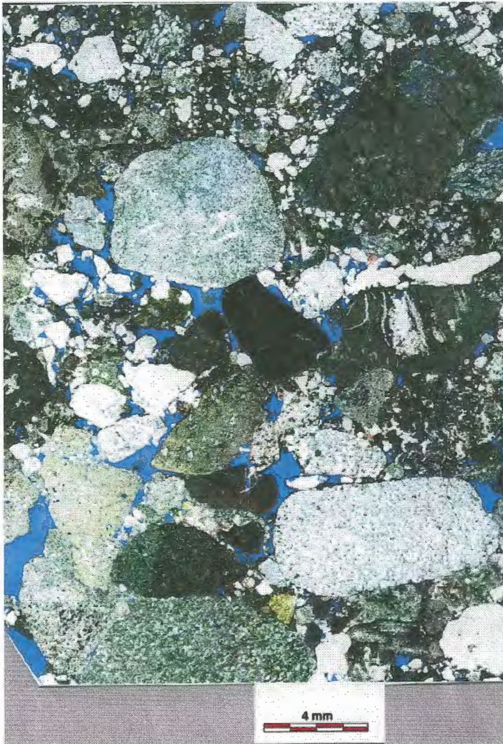
Figure 4.6 Intergranular porosity (unlikely to be primary because most of the Grantmire Formation shows evidence of dissolution) (Hunt Oil, 1998)
