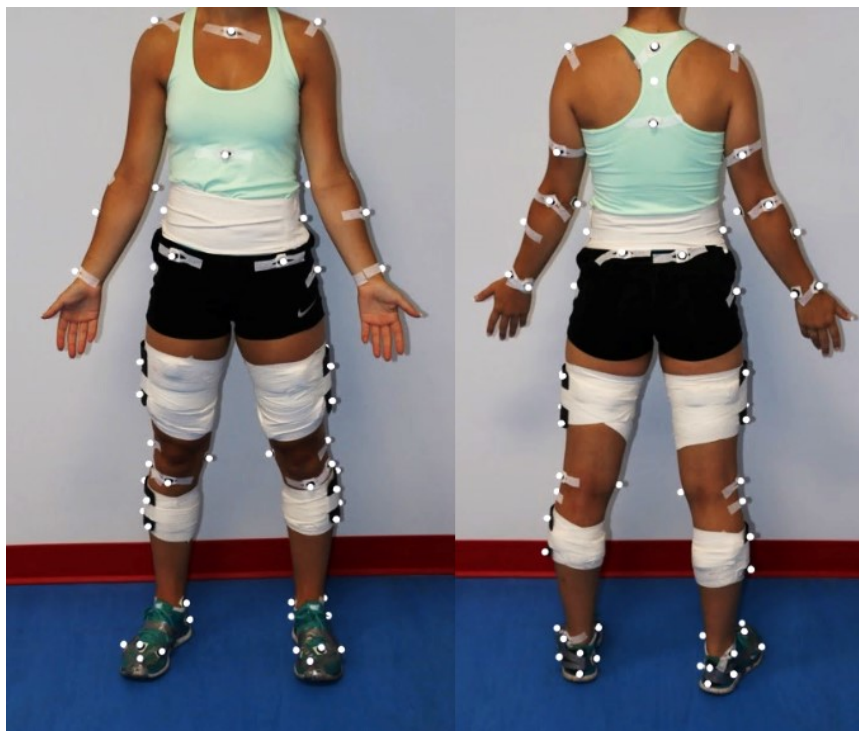
Figure 3.3. Retro-reflective marker placement on participant. Left: Anterior view; Right: Posterior view.
