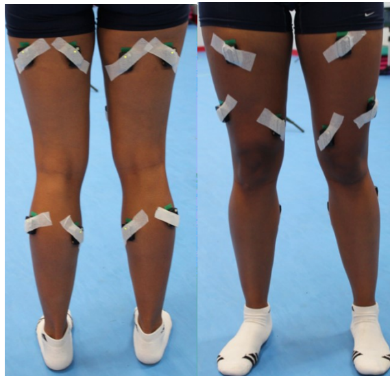
Figure 3.1. Electrode placement with Cover Roll on participant (Left: Posterior view; Right: Anterior view).
