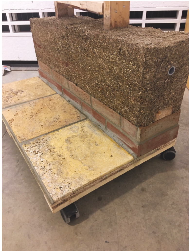
Figure 44: 1:1 Investigation - Hempcrete cast in place
