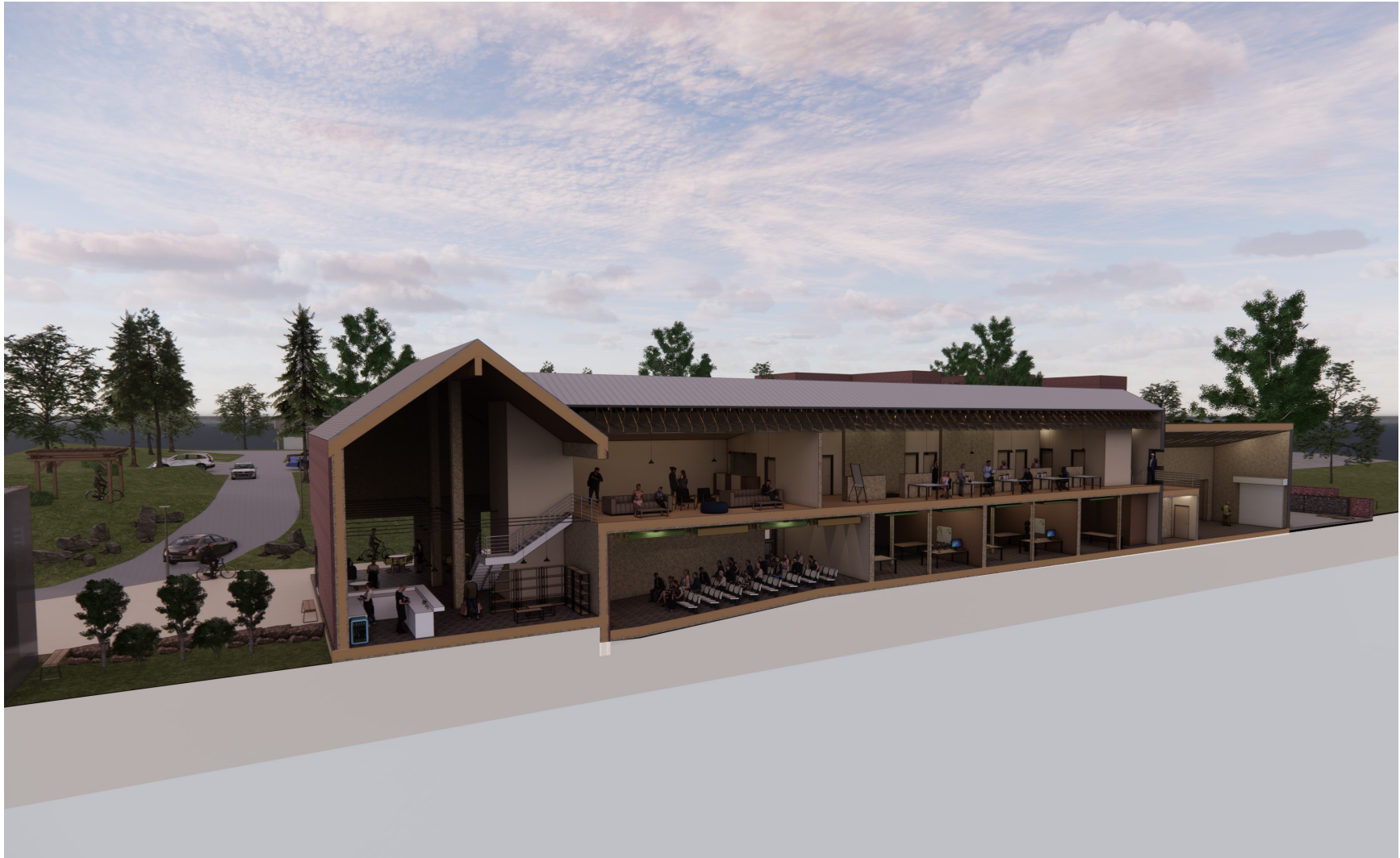
Figure 64: Inhabited Section: This is a section through the proposed Hemp Research Center at Dalhousie University in Truro, Nova Scotia. From left to right entering into the Hemps Cafe, then on the main level is the auditorium, labs, and workshop. Upstairs in the student lounge, studio space and workshop mezzanine.
