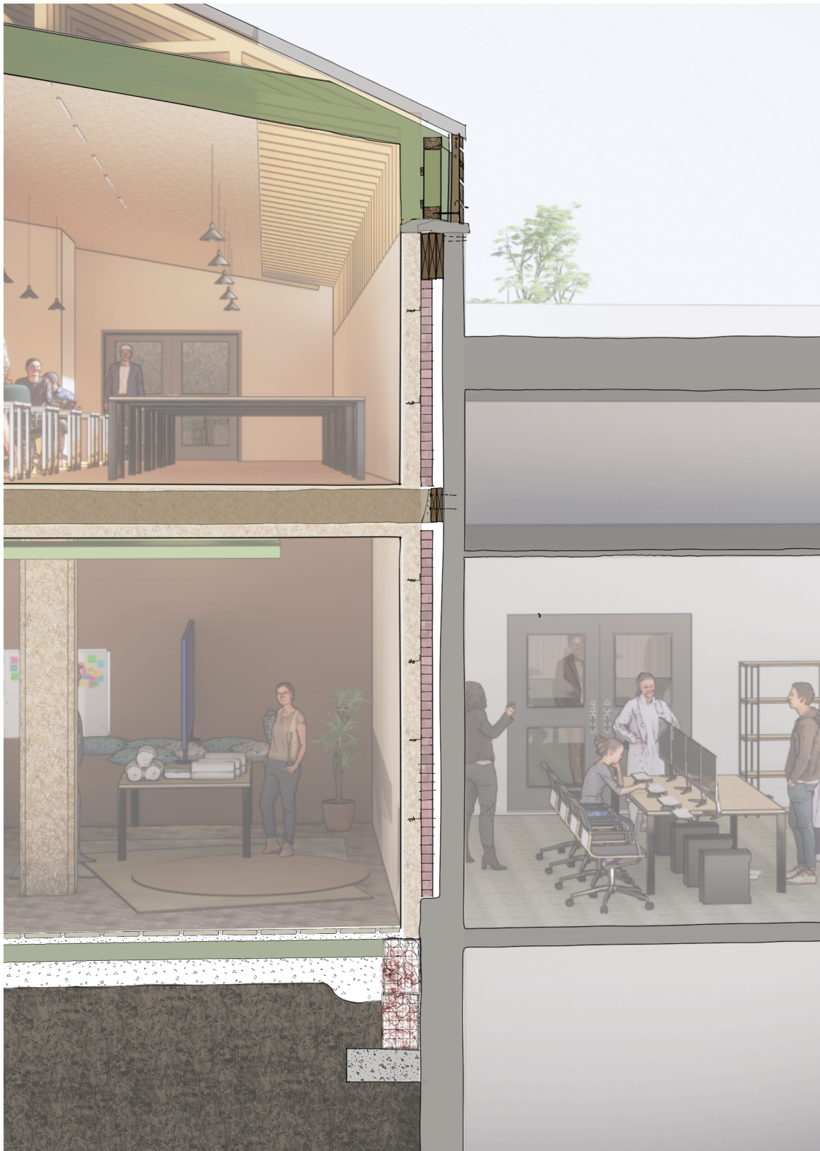
Figure 72: The shared demising wall between two buildings - In this section, the hemp textile lab shares a wall with an engineering lab. Offsetting the height of the new building allows sunlight to enter into the studio space.
