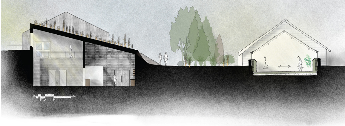
Figure 74: Cross Section relationship between the workshop and the existing greenhouse. The profile of the roof allows the sun full access to the green house year around.
