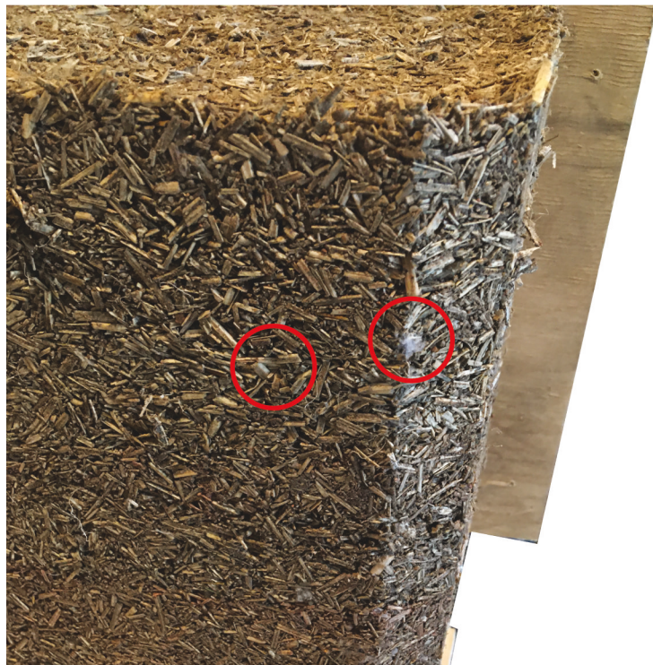
Figure 43: First hempcrete test resulting in mould spores due to moisture in the air and not removing the formwork at the appropriate time.
