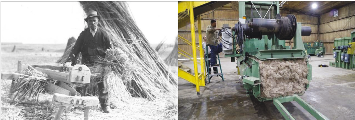
Figure 25: The image on the left is of a farmer separating the fibre from the woody core of the hemp plant using a tool that breaks the wood keeping the fibre strands intact. (Astre 2018). The image on the right is the modern-day version called a decordification machine that separates the two parts and bundles them into bales for use later. (Hemp Inc 2015).
