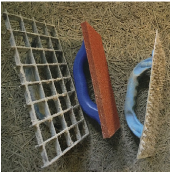
Figure 61: Grid, sponge, and nail floats: used for finishing planter and shaping hempcrete (Stanwix and Sparrow 2014, 107)
