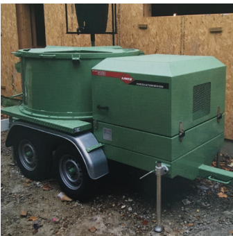
Figure 62: A large pan mixer is ideal for mixing hempcrete. (Stanwix and Sparrow 2014, 105)
