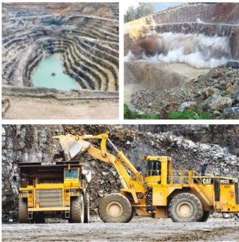
Figure 16: Quarry and mining processes to collect the components that make up cement. (Lion Bulk Handling 2020)
