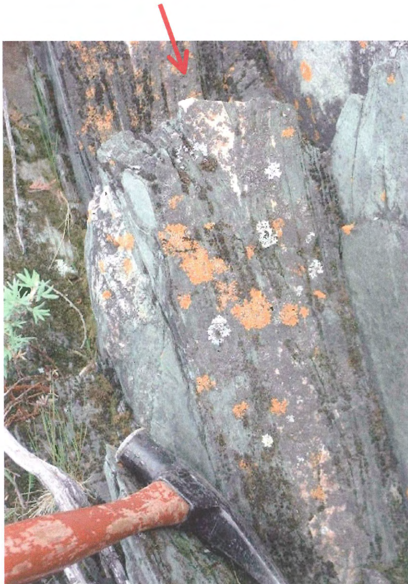
Figure 2.7 – Photograph from station 8 showing steeply dipping foliation. A small granite vein is boudinaged in both the horizontal and vertical direction. This photograph shows the vertical dimension.
