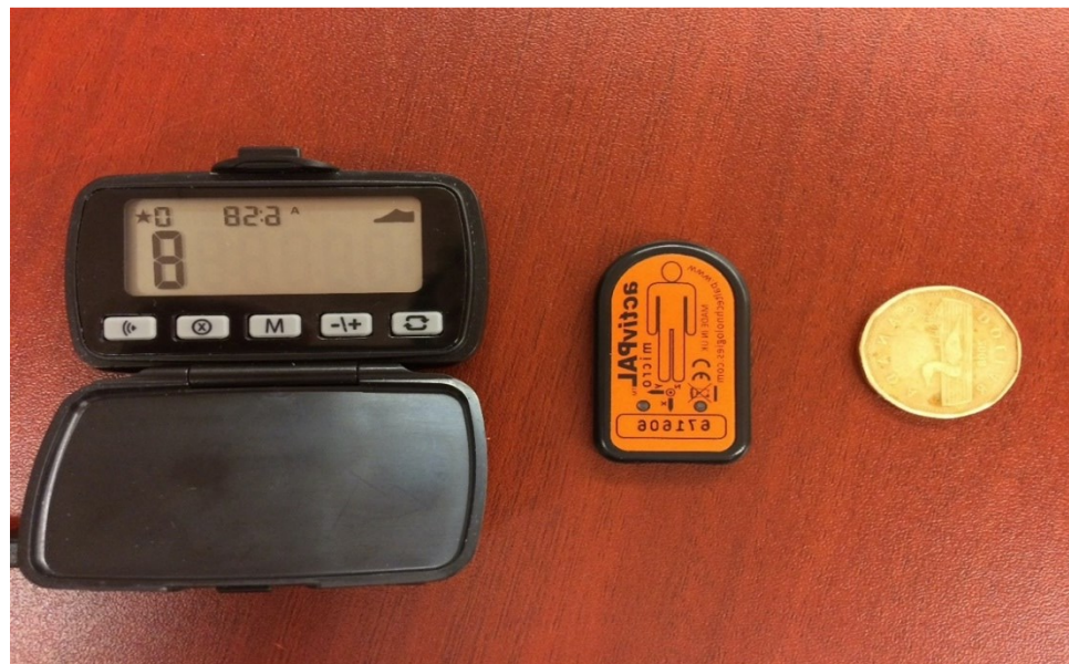
Figure 2-12: The activPAL™ and PiezoRx®, placed beside a one dollar coin for size reference. The activPAL™ will be placed anteriorly on the mid-thigh. The PiezoRx® will be worn on the waist or belt in accordance to manufacturer recommendations.
