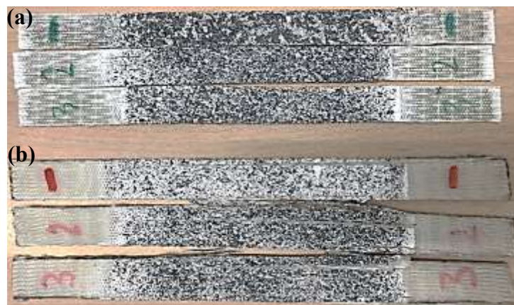
Figure 3-4 FRP coupons after reaching their ultimate tensile stress capacity; (a) GFRP coupons; (b) PET FRP coupons.
