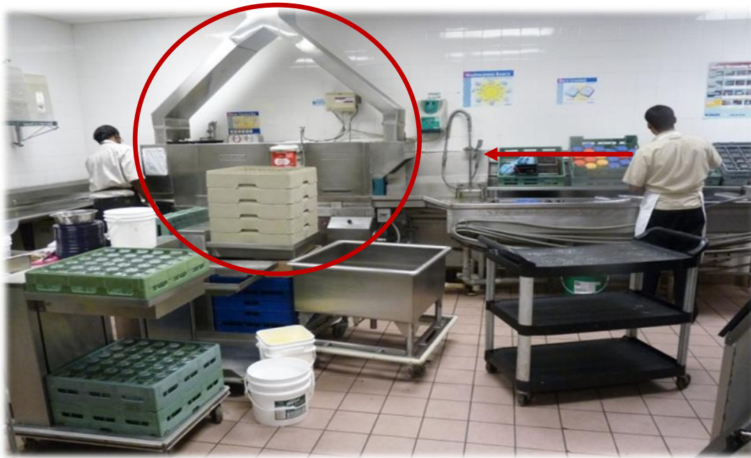
Figure 1: Howe Hall's Dish-pit. The arrow points to the sprayer, the dishwasher is circled.
