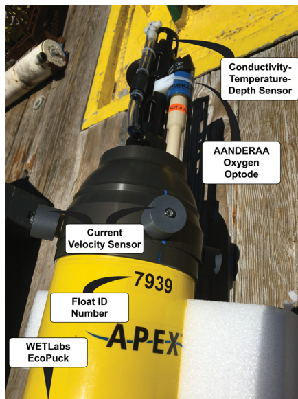
Figure 3.1: Photo of float f7939, one of the 10 autonomous EM-APEX floats with the various sensors labelled.
