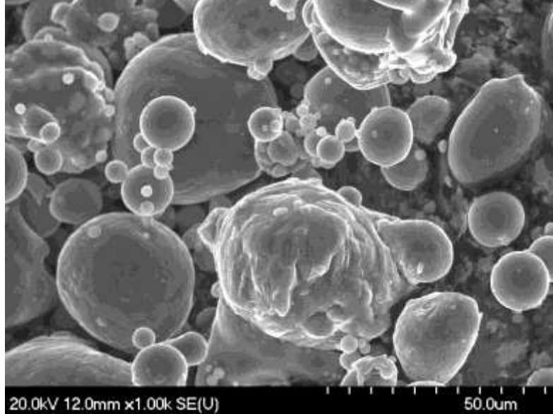
Figure 4-1 SEM image of Al-0.3Sc-0.2Zr gas atomized powder.
