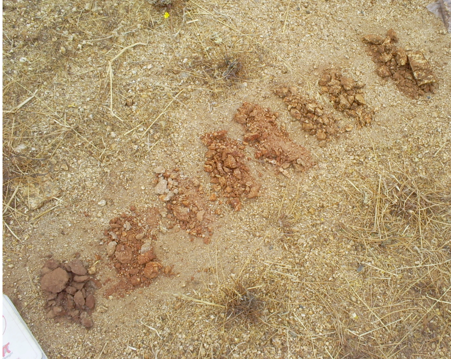
Figure 3.2 Rock samples laid out on the ground where the upper right corner represents the base of the profile (8.29 m from surface) and the bottom left represents an upper sample. (photo by J. Gosse, 2007)
