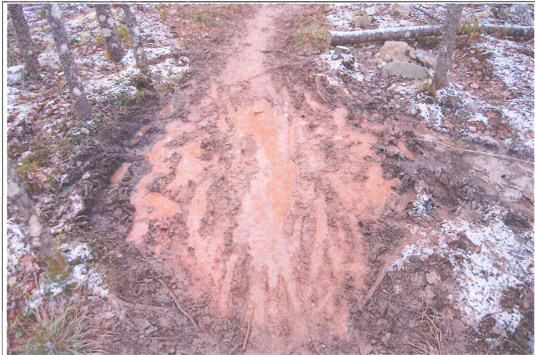
Figure 3.3. Visual effect on the trail-bed from biking and walking. Bike ruts a generated along and near to the trail axis. Trail widening by boot prints are also visible at the edges of this wet depression. This photograph, because it is at a wet transect, shows the greatest effects of both users.
