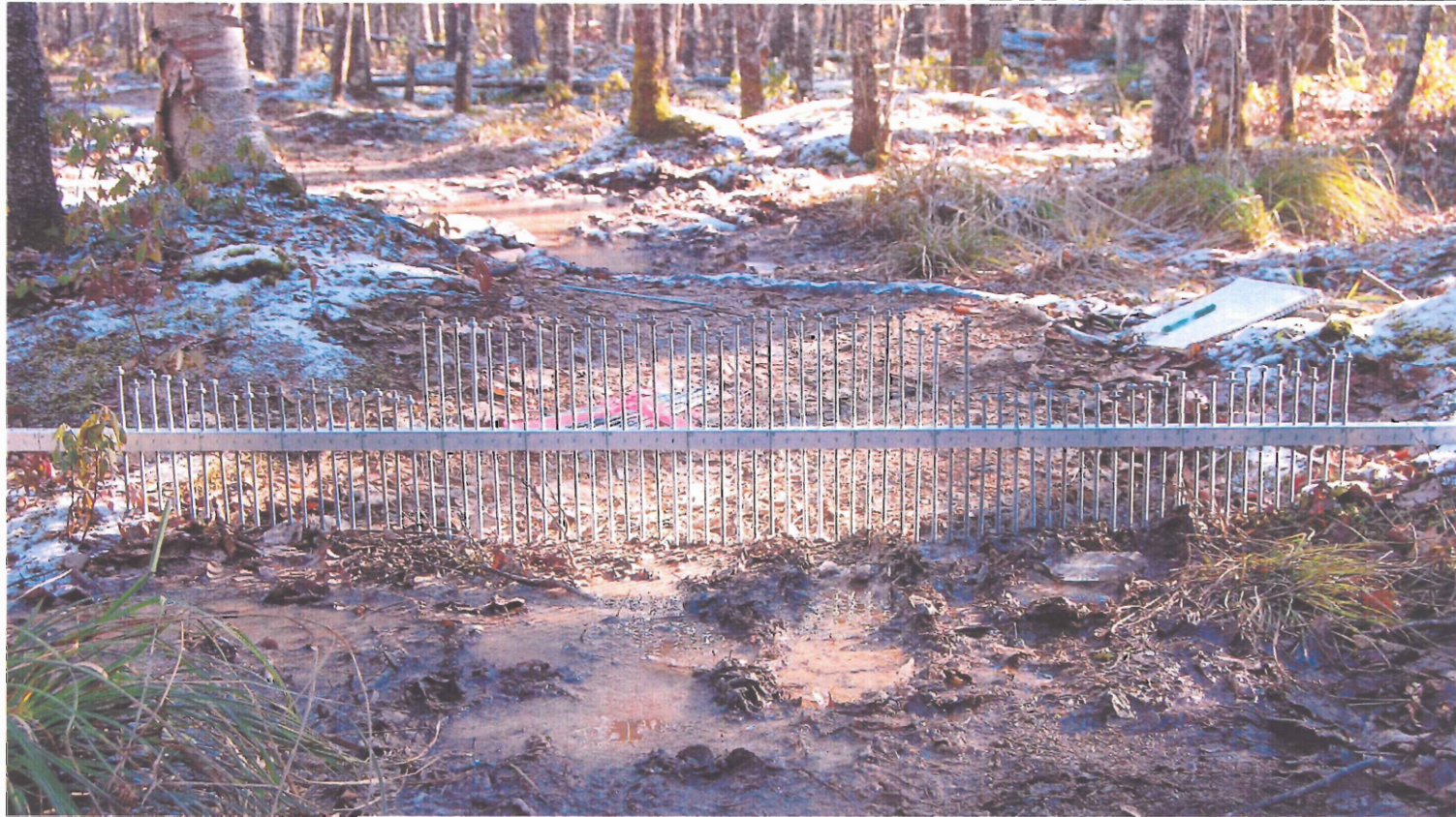
Figure 2.1. Photograph of LT-Device being used on the trail (the long rods in the center are 30 cm in length, the shorter rods at the ends are 20 cm)
