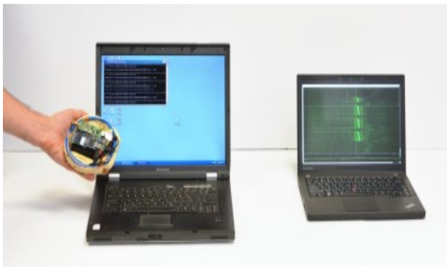
Fig 3. 2 Schematic diagram of the measurement process. The PITA first measures the target computer (left) at a specific frequency band and then transmit digital signals over Wi-Fi to the attacker's computer (right) in real time.[19]
