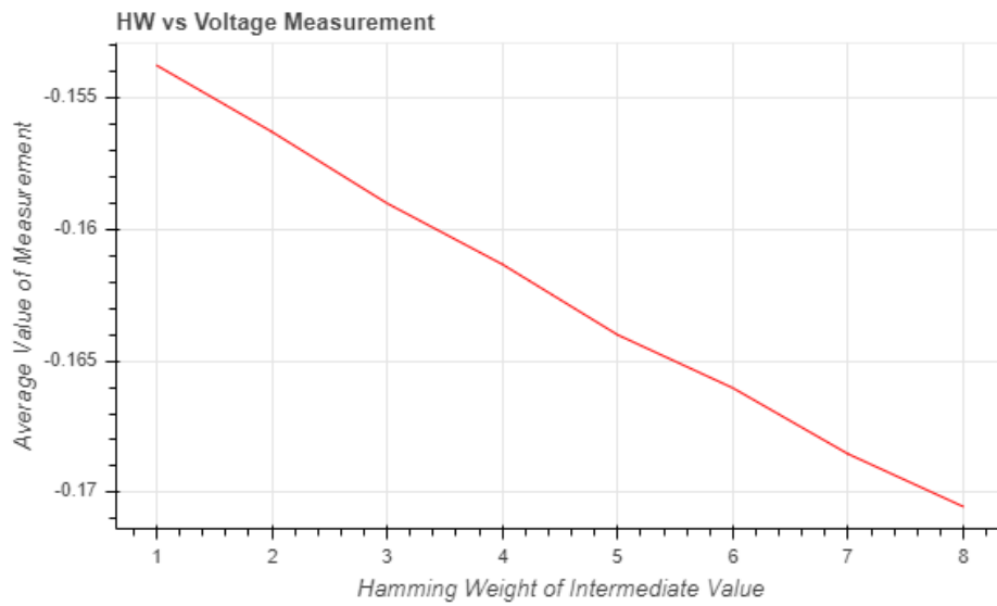
Figure 4-23. HW vs Power Consumption, STM32F071
