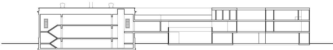
Building section D: cutting through the community gym, childcare centre and W.S. Feilding building
