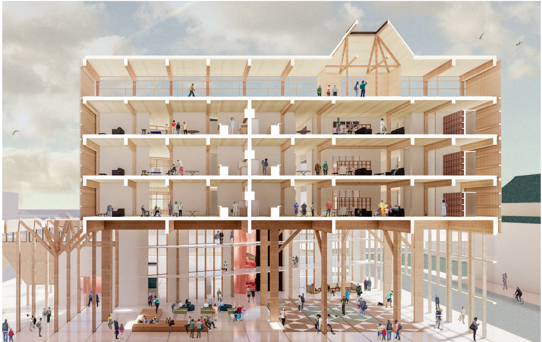
Section perspective through the retail plaza, the multi-generational housing, and the town hall.
