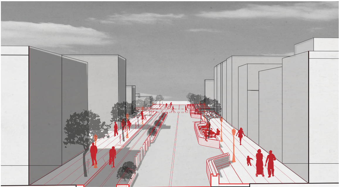
Van Brunt Street – Section. A consistent set of design elements (bike lanes, widened sidewalks, vegetation, and lighting) can improve the pedestrian and cyclist's experience of the street. Heterogeneous program elements enable adjacent uses to integrate and benefit from the new street infrastructure.
