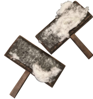
Carding brushes from the Nova Scotia Textile Mill used to comb raw or washed wool into straight fibres in preparation for spinning. (West Hants Historical Society, 2018).
