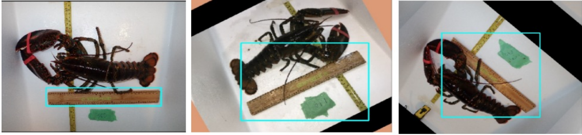
Figure 4.1: Detecting axis-aligned bounding boxes around the ruler in the image. Axis-aligned bounding boxes do not tightly fit the ruler when it is at an angle to the horizontal in the image.
