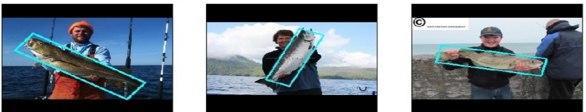
Figure 3.2: Rotatable bounding boxes are a tighter fit for the object of interest and thus a better measure of its dimensions.
