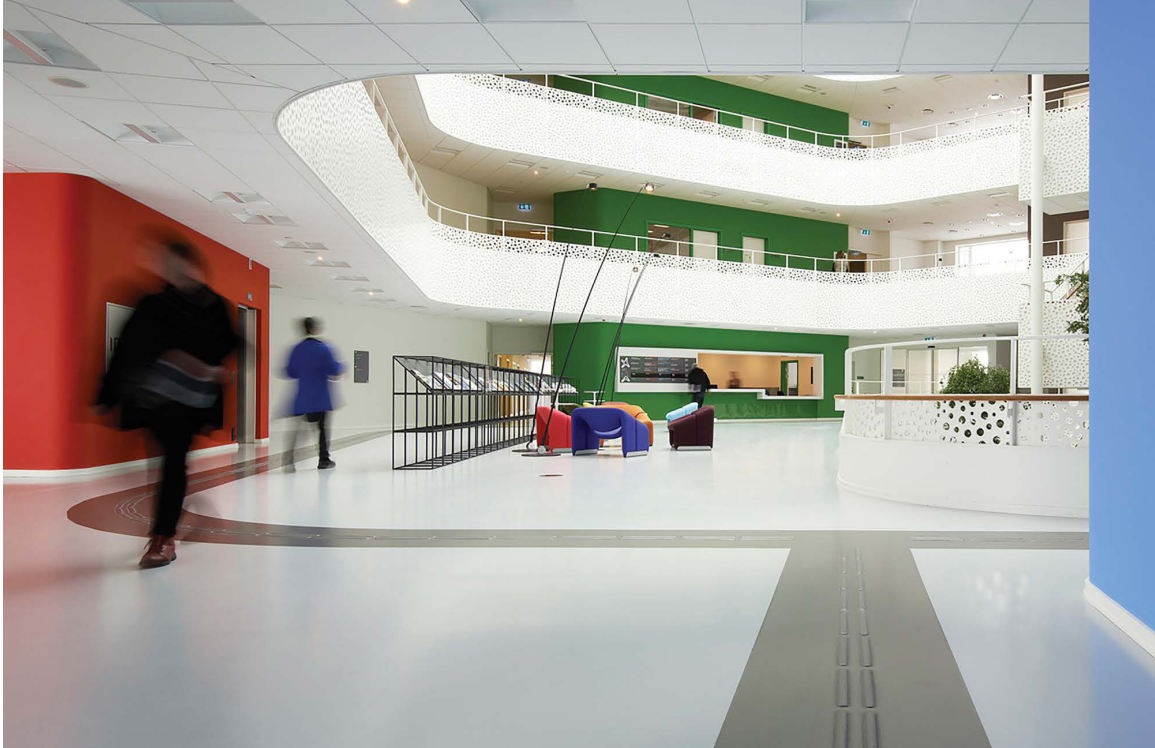
Cubo & Force4 Architects, Danish Handicap House atrium. Note the inset elements for cane-based navigation and the color coding of each wing. (Force4 n.d.).
