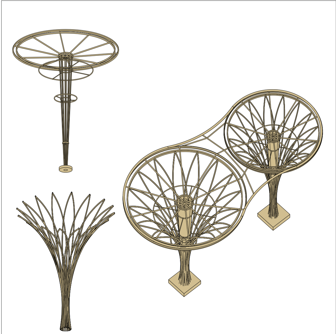
Movable bamboo roof structures: these structures are meant to provide shading and create inhabitable spaces for people.
