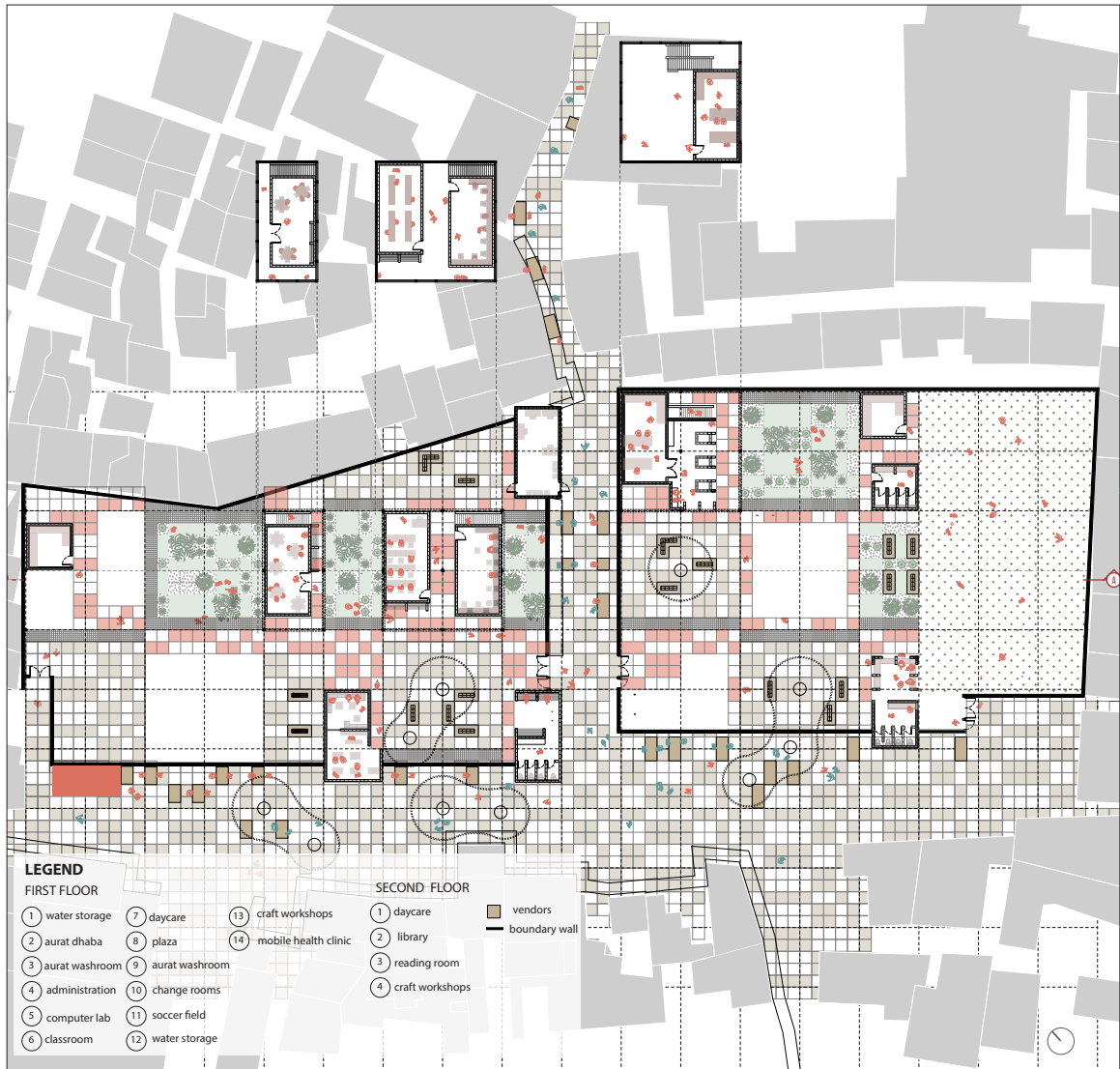
Phase Two-Revitalize: level 1 and 2 floor plan.
