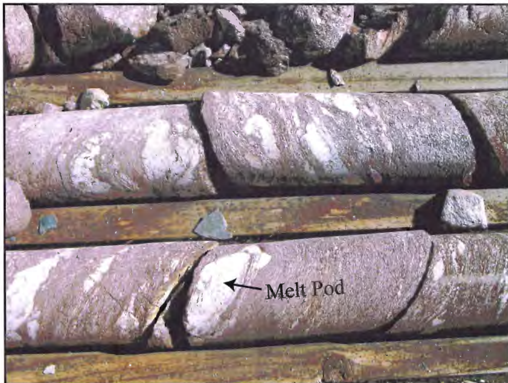
Figure 3. 11: HLMC core samples retrieved from Cameco core box on Fenwick Lake, Leith Peninsula. Cores are highly hematized, evident by the rusty coloration. Melt pods abundant with foliation defined the alignment of phyllosilicates.
