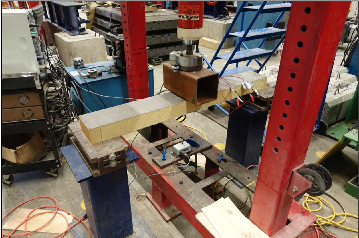
Figure 3: Static Three-point Bending Test Set-up – Courtesy of Dillon Betts
