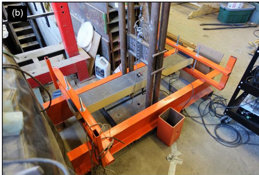
Figure 2: Impact Test set-up (a) schematic (b) lab photo – Courtesy of Dillon Betts
