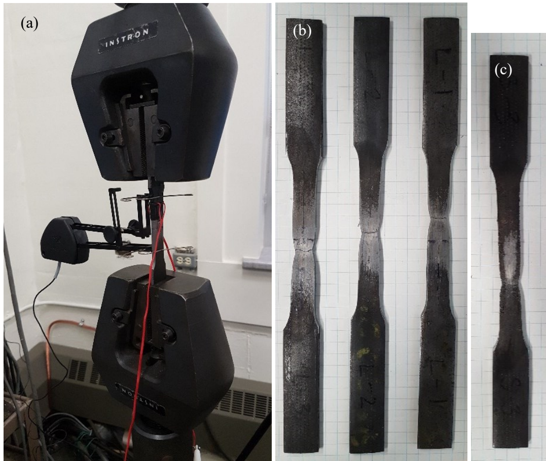
Figure 3-4 Steel tension testing: (a) test set-up; (b) tested specimens L-1, L-2 and L-3; and (c) tested specimen S-3.
