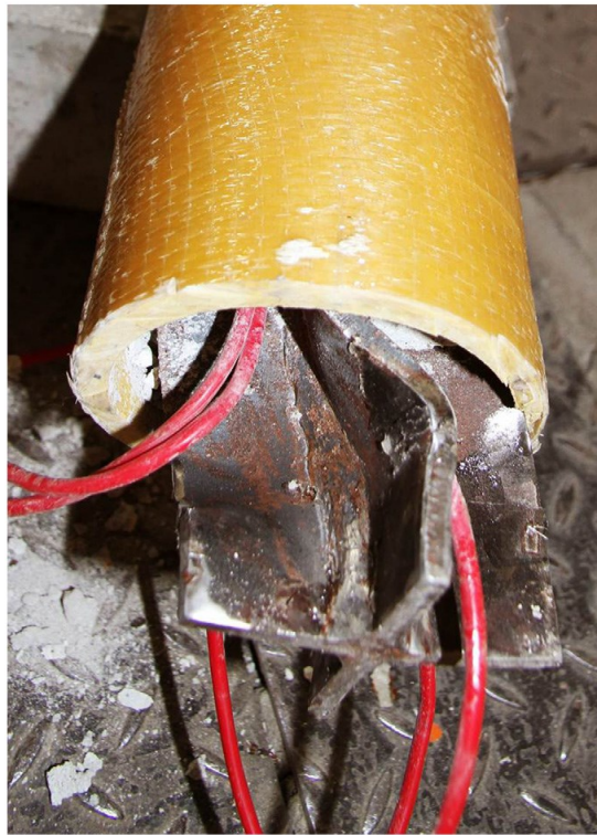
Figure 2-16 Cross-shaped specimen showing local buckling at ends (Feng et al. 2013)
