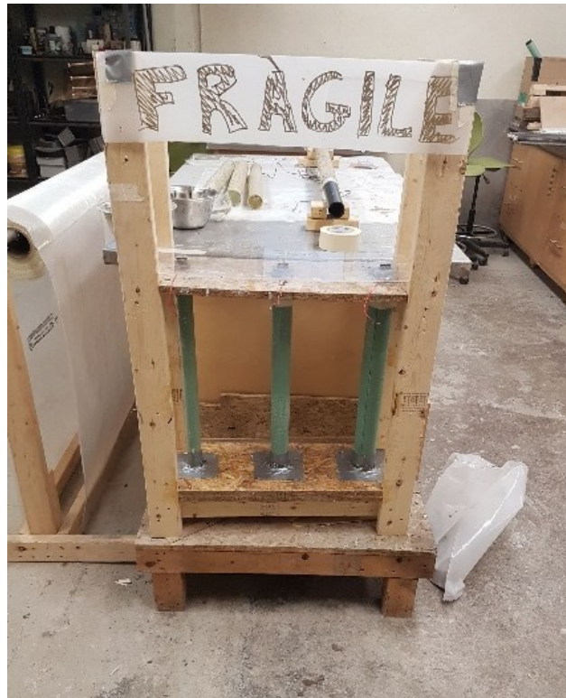
Figure 3-8 FRP-BRB casting frame
