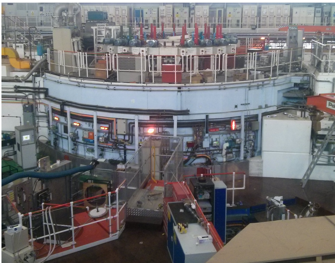
Figure 3.7: The ISIS neutron source. Displayed is the containment structure of the tungsten target from which neutrons are produced. For scale, see the ladder on the right of the image. The sample access port of the GEM detector can be observed in the bottom right.
