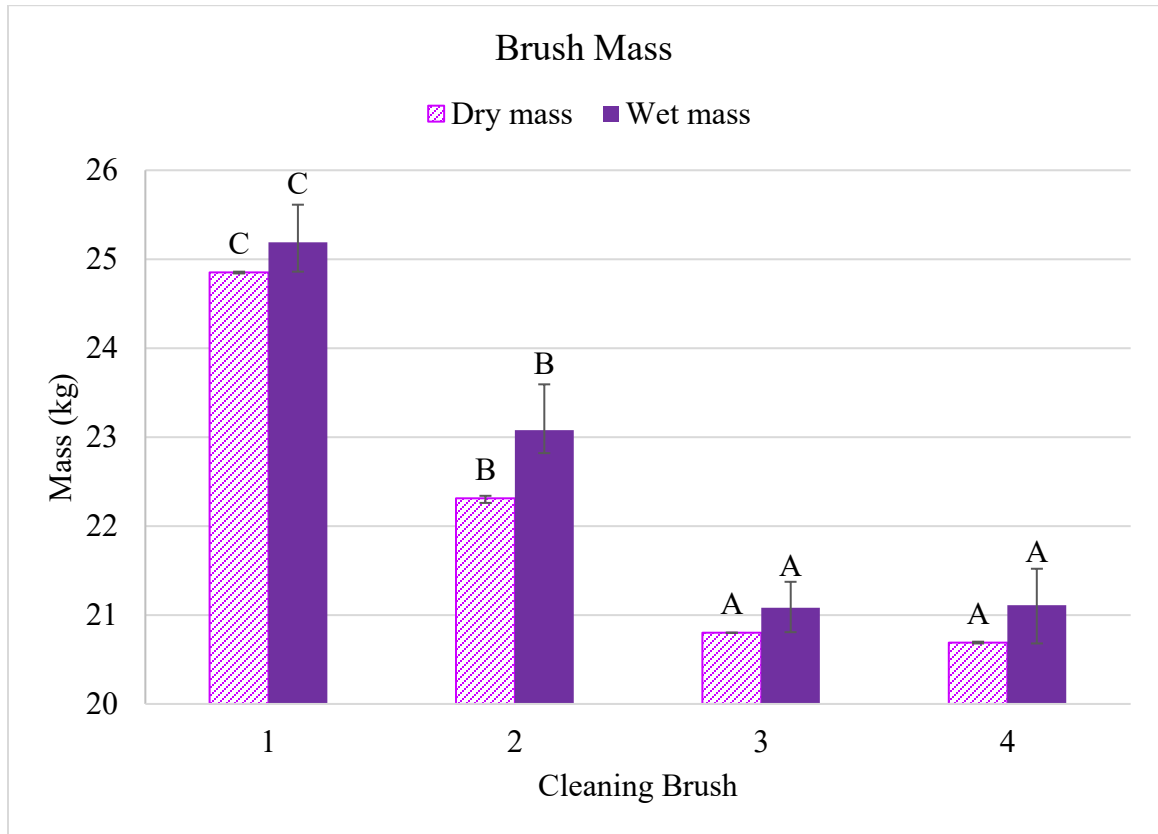
Figure 3-18: Mean comparison of debris cleaning brush dry and wet masses. Error bars represent the minimum and maximum masses from the repeated sampling measurements on each brush.
