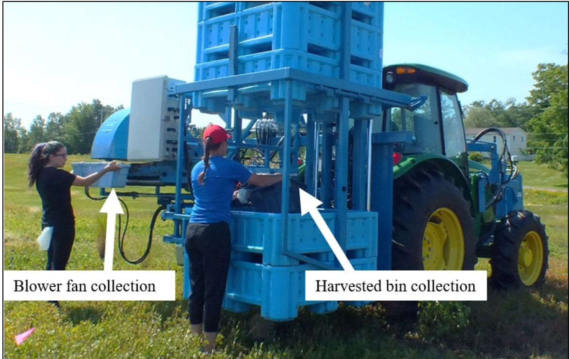
Figure 2-5: Field data collection from mechanical wild blueberry harvester blower fan and bin.
