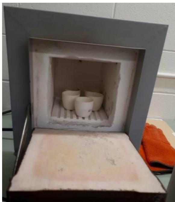
Figure 3-5. Furnace used to combust samples 001 - 006 at 450 °C for 5-6 hours to remove carbon material from sample (Soukup, 2017).
