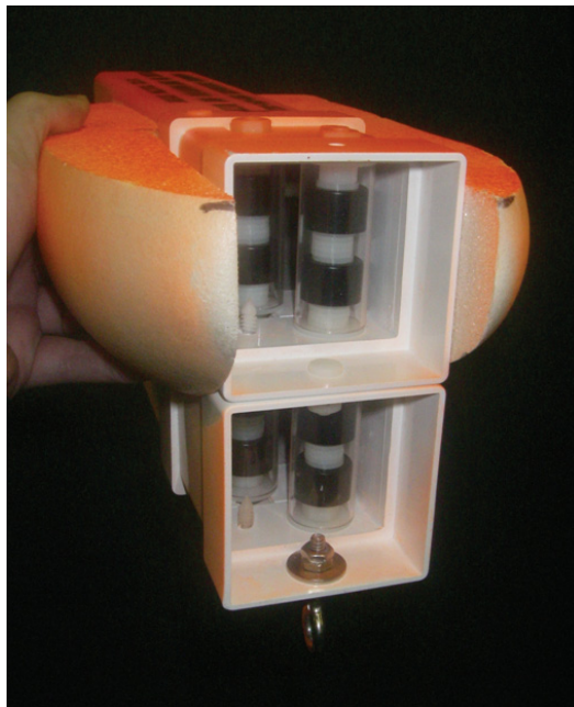
Figure 2.3 Leading-end aperture image of a magnetic-collector designed to capture near-surface and sub-surface magnetically attractive particles (MAPs). Rare-earth magnets within their encasement tubes are located within the aperture, floatation nacelles are attached to the upper tube, and the mooring attachment is located on the lower tube.
