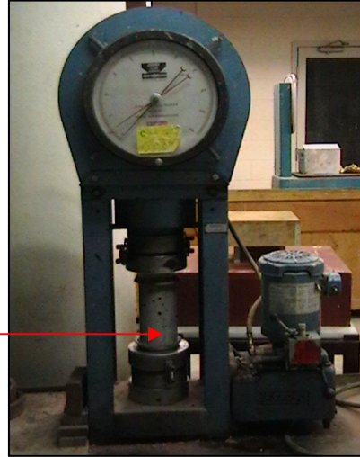
Figure 4.4 Compression testing machine
