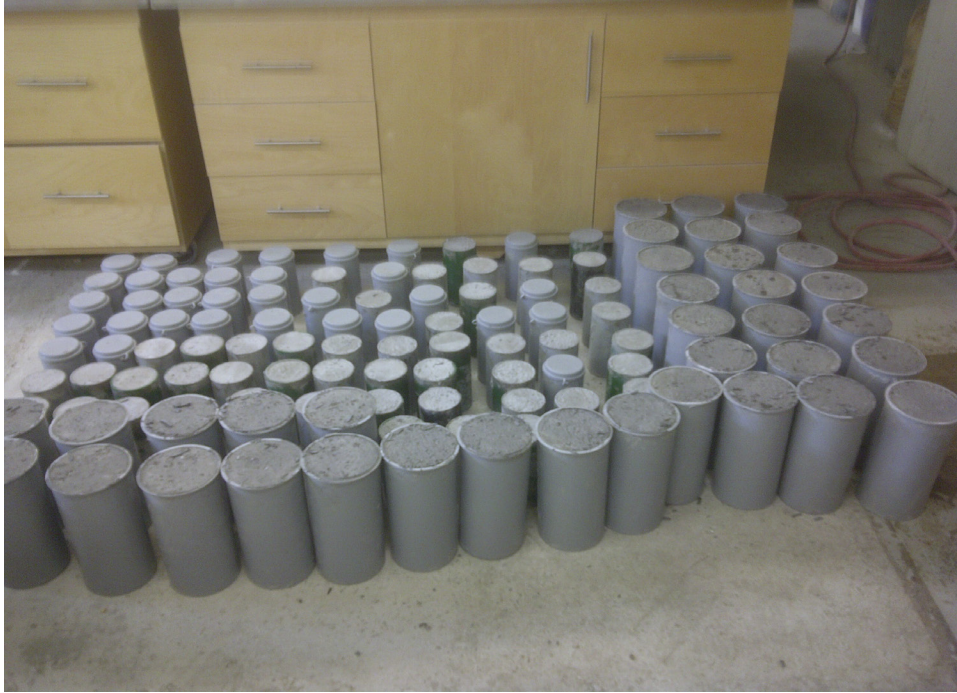
Figure 4.3 Concrete cylinders prepared and cast in the laboratory
