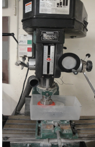
Figure 4.6 Milling machine used to grind-test concrete specimens
