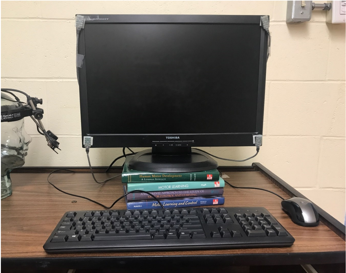
Figure 3.3. Experimental setup as viewed by the participant including display monitor with infrared targets for Eyelink II system and keyboard.
