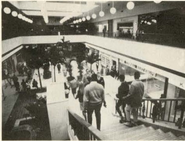
Interior of the two-level Colonie Mall at Albany N.Y. Open floor allows shoppers to view stores on both floors. Lower level stores are extended forward to edge of upper walk. Upper walk is usually 12 to 15 feet wide.
