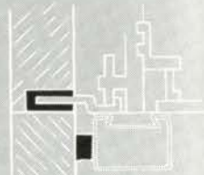
WEATHERPROOFING JOINTS BETWEEN METAL AND STONE
