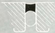
SEALING JOINTS IN STEEL PANELS
