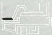
CAULKING SASH PERIMETERS
