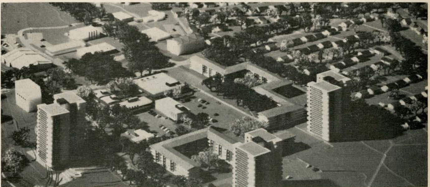
OTTAWA: CMHC and the Ontario government retained the town planning firm of Project Planning Associates to prepare designs for a large suburban housing site, Borden Park. Design shows family neighborhoods clustered around a small Town Centre, with parks and community buildings. High-rise rental housing is placed close to the centre, so shops and public transportation will be accessible to single and older persons
