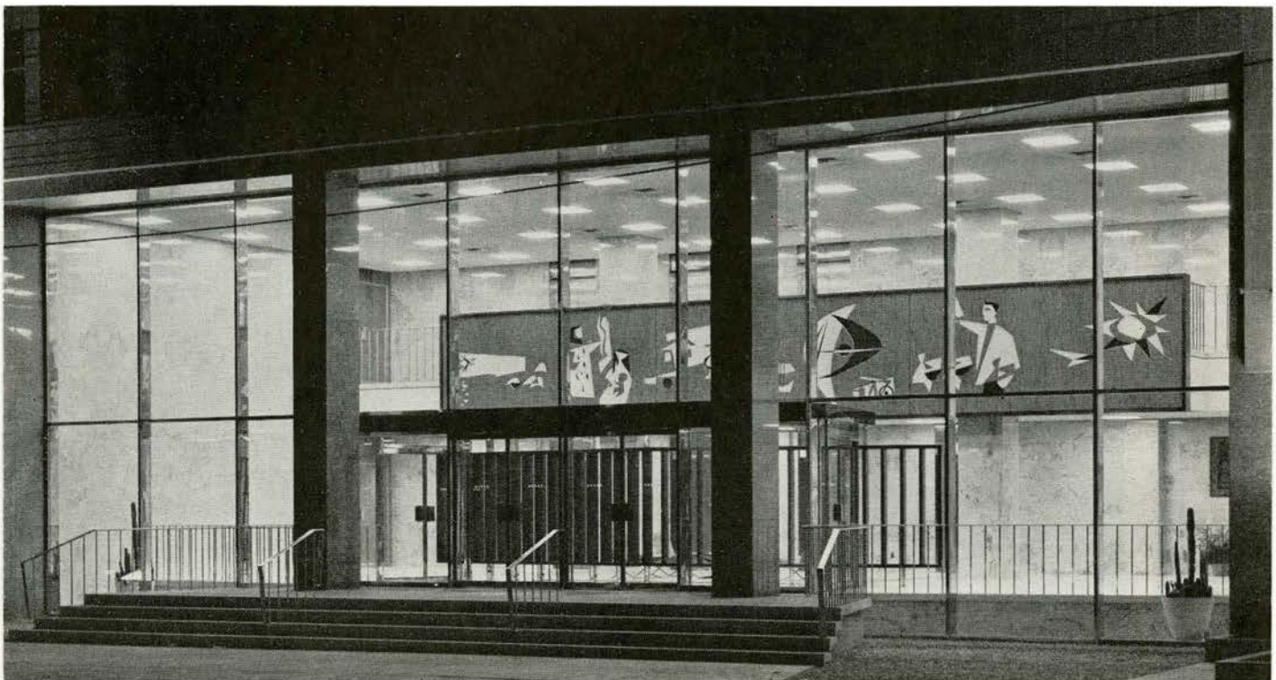
Above: The foyer at night, showing the mural by Stefan Fritz. Sgraffito. (Three layers of 1/4" coloured plaster, black, natural and terracotta. The design is carved through the layers to expose the colours.)
