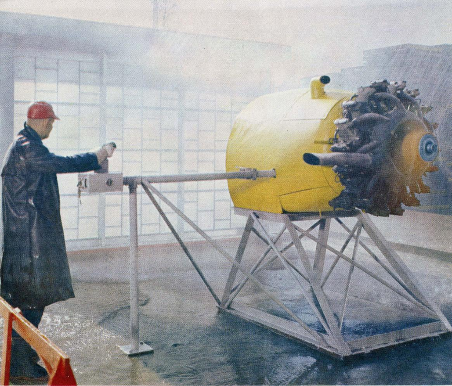
Aircraft engine hurls gallons of water against THINLITE wall at near-hurricane velocity in weather-resistance test.
