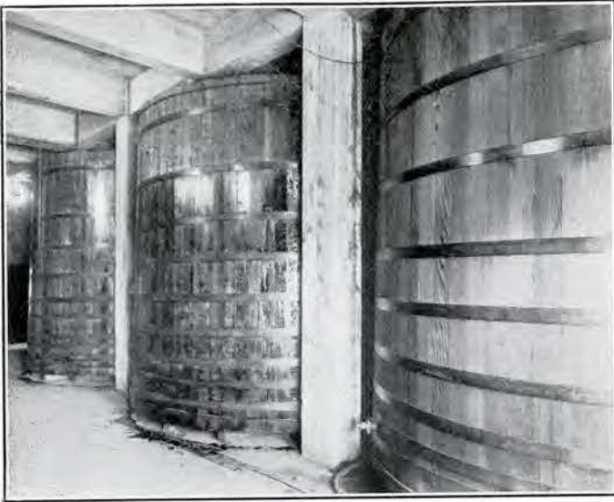
Close-up view of California Redwood Tanks built and installed by the Ontario Wind Engine & Pump Co., Limited for an Ontario Winery.
