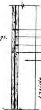
Construction: 8.2. 1" Drop Siding Tar Paper. Building Paper Shiplap. 6" Studs.
