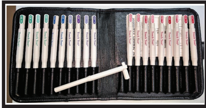
Figure 2.7 von Frey Hair Filaments (Left to Right – Increasing Bending Force)
