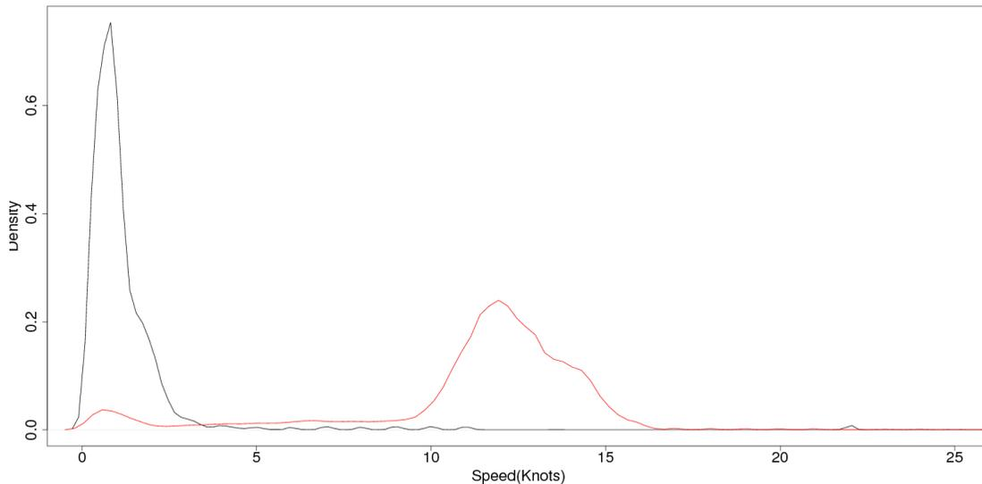
**Fig. 2.4 Speed distribution for purse seiners.** The red line indicates the probable non-fishing activity labeled by the expert, while the black line represents probable fishing activity. This distribution considers only the speeds reported by the vessels more than 10 km from shore and during day time
