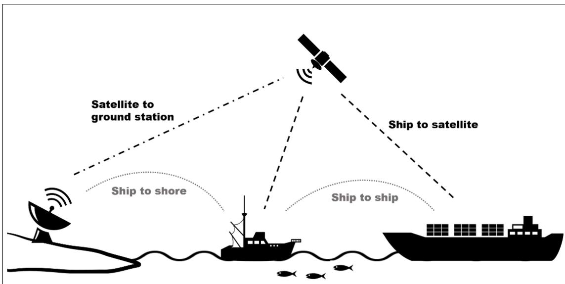
**Fig. 1.2 Scheme of Automatic Identification System (AIS) signaling between ships carrying the transponder as well as satellite and ground stations.**
