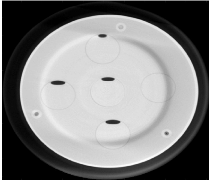
Figure 3.9: Crescent artifact for 140 kV, 2000 mAs, full-fan bowtie half-arc acquisition, resulting from improper crescent calibration.
